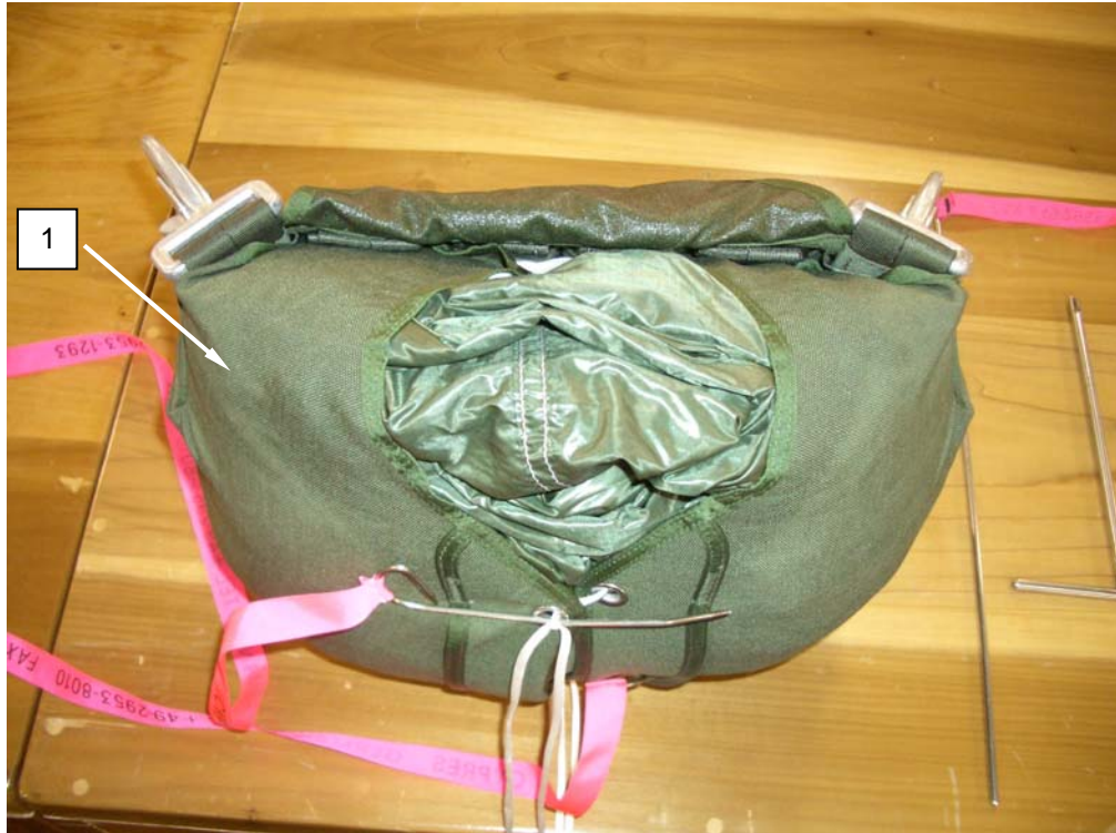
Figure 48. Tucking Left and Right Sides into Pack Tray.
