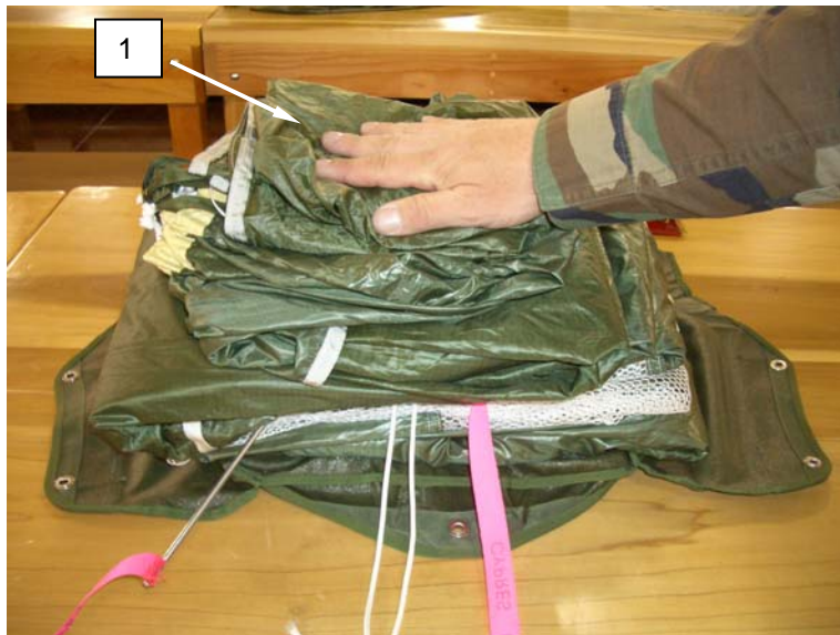
Figure 44. Centering Extractor on Top of Folded Canopy.
