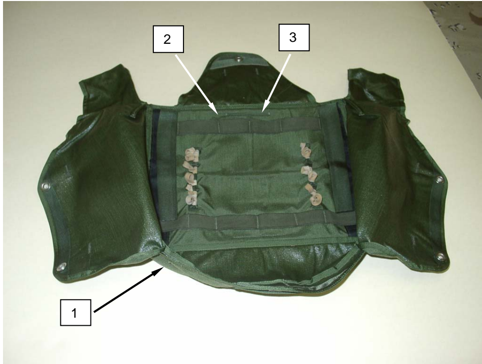
Figure 1. Remove Damaged Elastic Riser Stow Bar.
