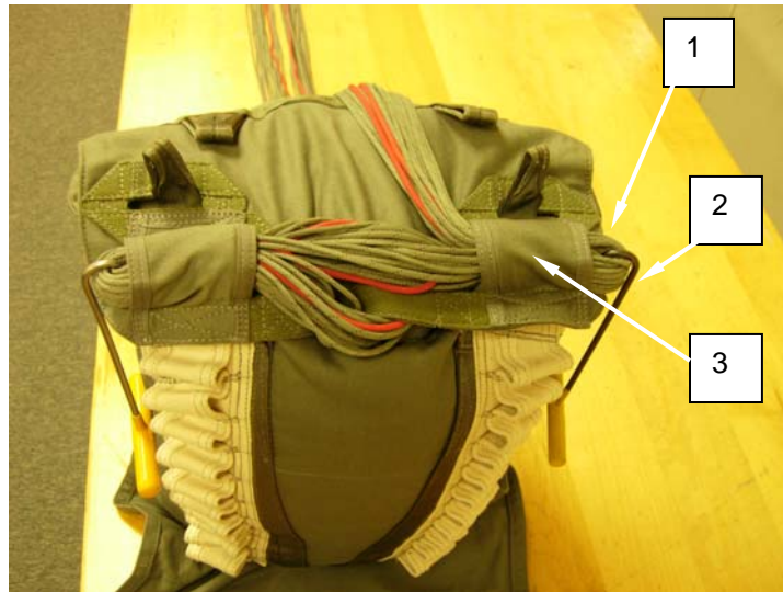
Figure 52. Closing Deployment Bag and Stowing Suspension Lines (continued).
