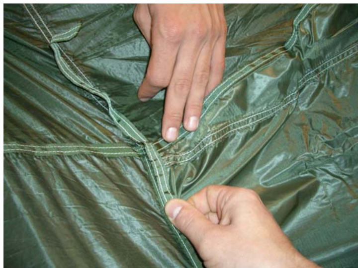
Figure 4. Aligning New Extended Gore with Open Gore.
