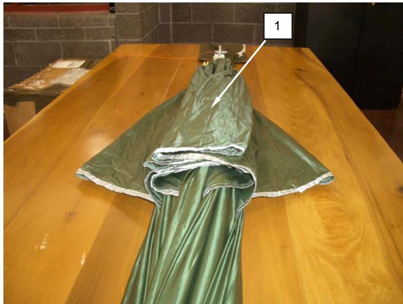
Figure 19. S-Folding Left and Right Side on top of the Folded Top Apex Scoop.
