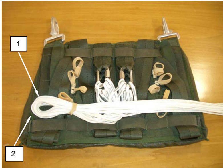
Figure 27. Making First Regular Stow.
