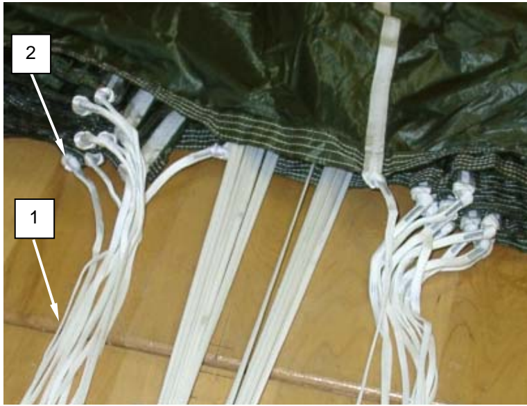
Figure 1. Attaching New Suspension Line To Attaching Loop.
