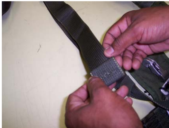
Figure 8. Replacing Harness Left Upper Main Lift Web (continued).
