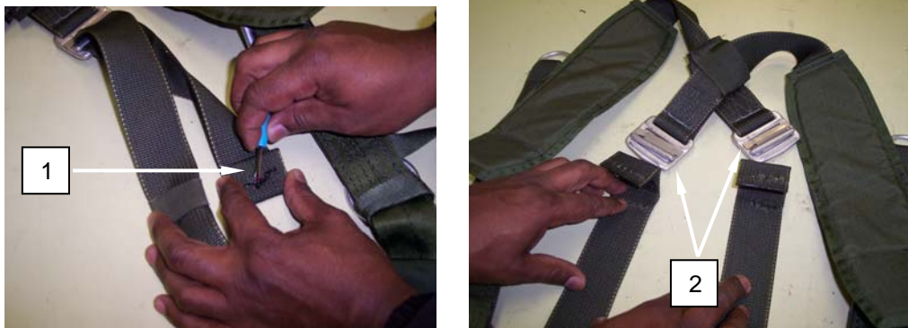
Figure 1. Replacing the Saddle Assembly.
