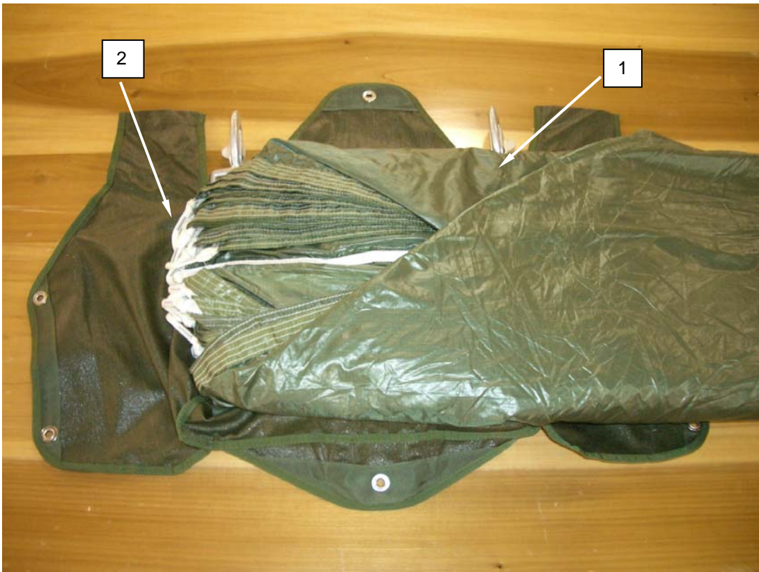
Figure 36. Placing Canopy into Pack Tray.
