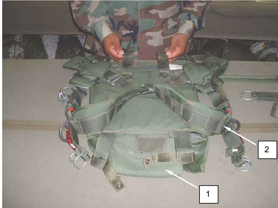
Figure 5. Attach Harness To Pack Tray.
