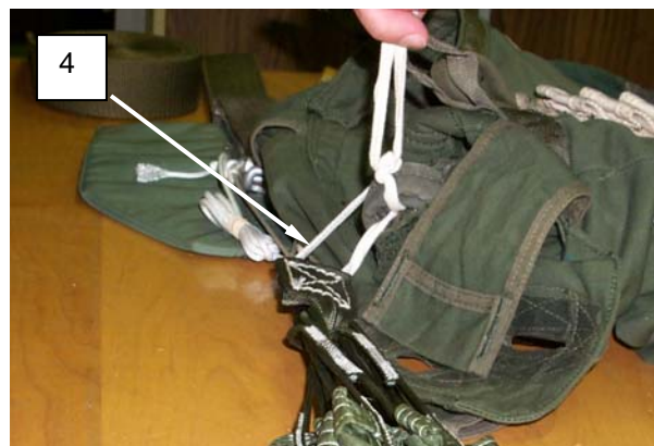
Figure 44. Securing Main Canopy Vent Loop to Girth Hitch of Static Line.
