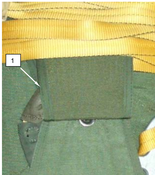
Figure 1. Replace Damaged Pin Protector Flap.
