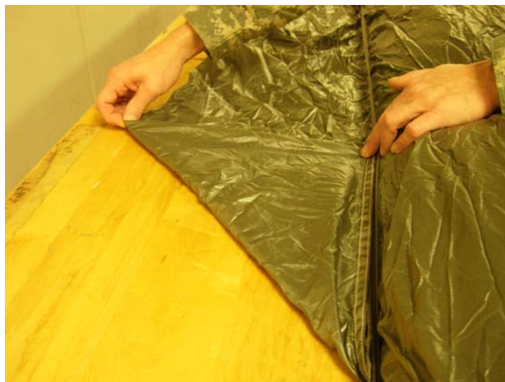
Figure 41. Gore 13 Slot Folded to Radial.
