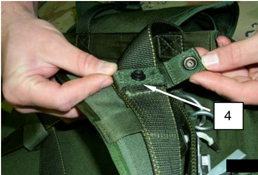
Figure 3. Route Small Tuck Tab, Close Snap Fastener, and Snap Fastener Secured.
