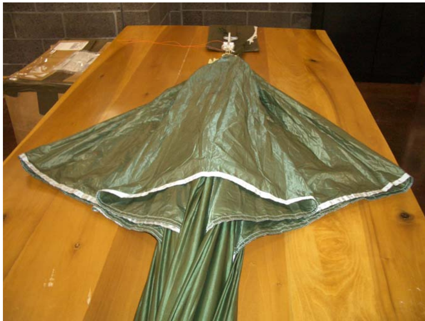
Figure 12. Folding and Dressing Left and Right Apex Scoops.
