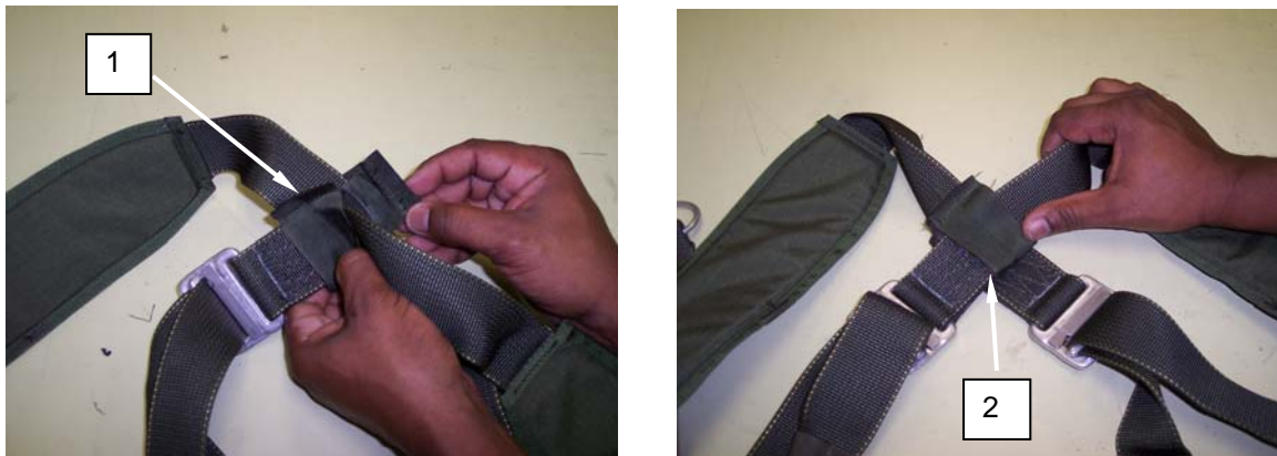
Figure 7. Replacing Harness Left Upper Main Lift Web (continued).
