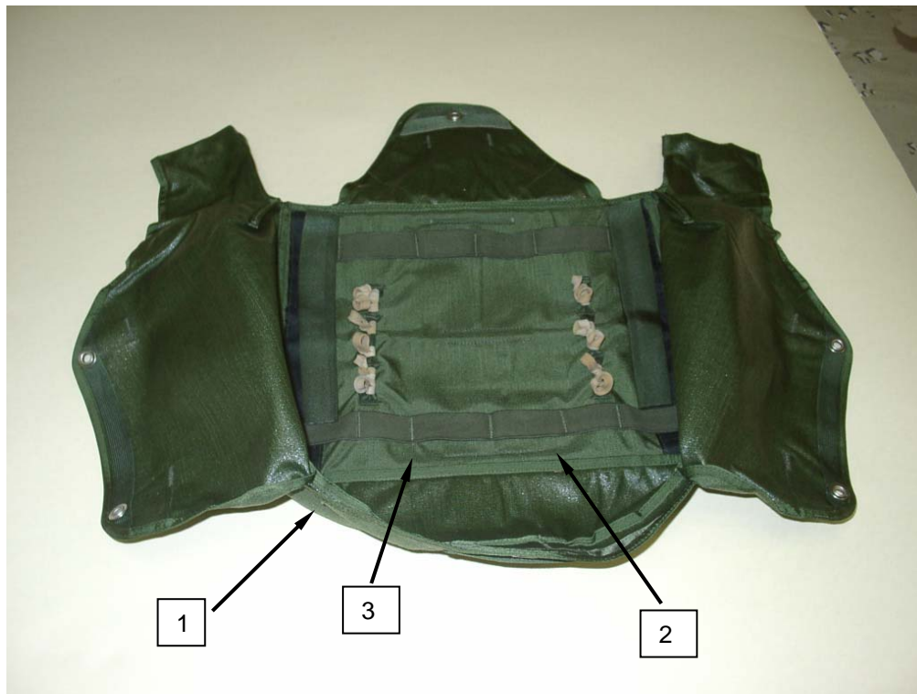
Figure 2. Replace Lower Elastic Riser Stow Bar.
