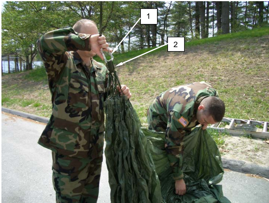
Figure 1. Connecting Snap On Pulley Rope to Canopy Bridle Loop.
