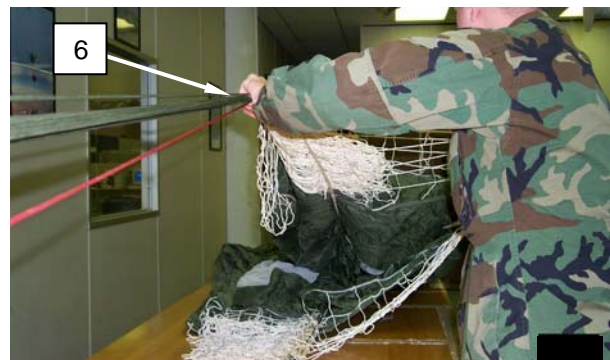
Figure 18. Aligning the Upper Lateral Band and Folding the Gores.
