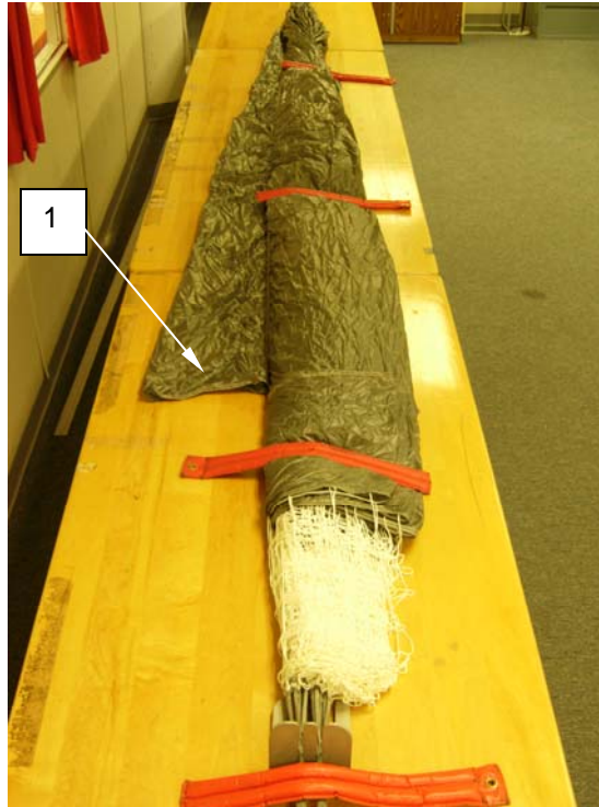
Figure 40. Gore 13 Slot Unfolded.
