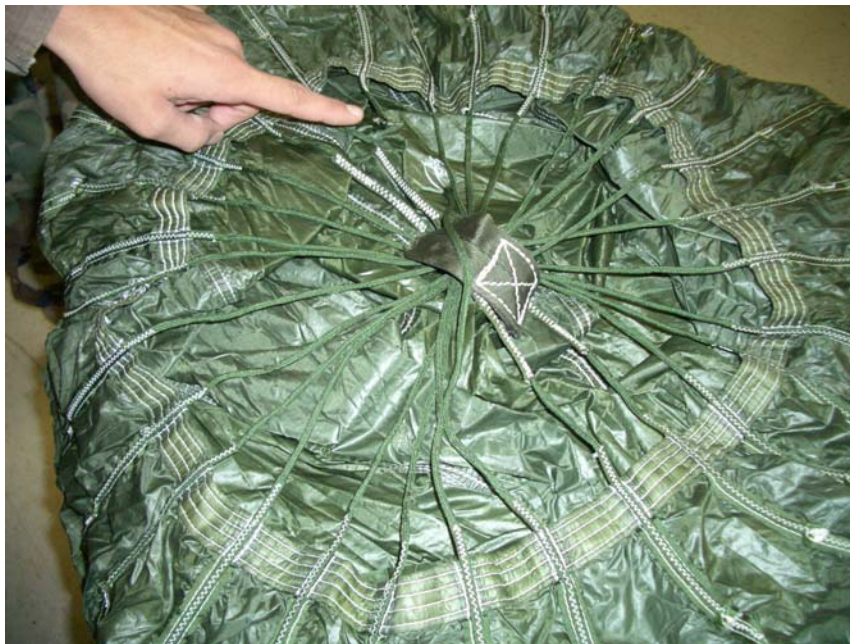
Figure 1. Main Canopy Vent Line Repair.
