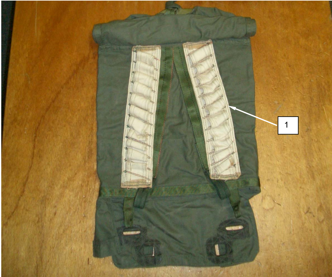
Figure 1. Replace Suspension Line Stow Loops.
