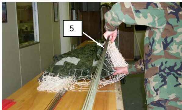
Figure 18. Aligning the Upper Lateral Band and Folding the Gores.
