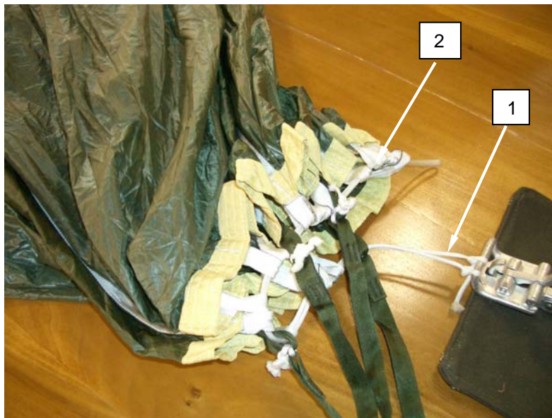
Figure 4. Passing Apex Hook-up Lanyard thru all Apex Loops.
