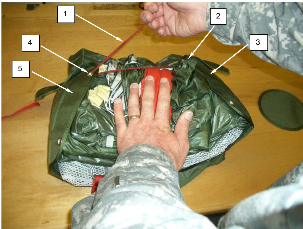
Figure 45. Placing Lower Pull Up Cord thru Lower Grommet.
