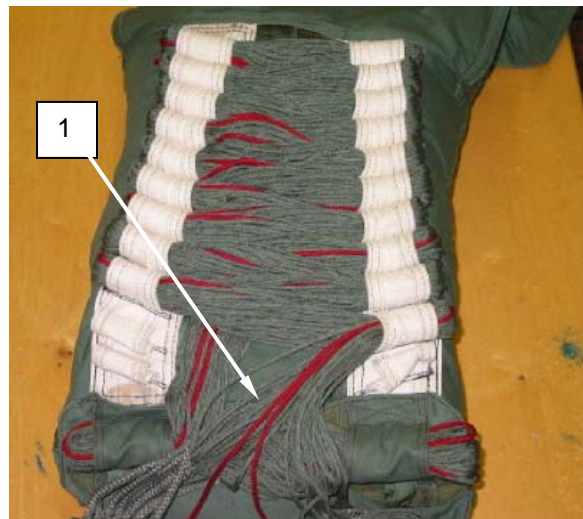
Figure 55. Continuing to Alternate Stows.
