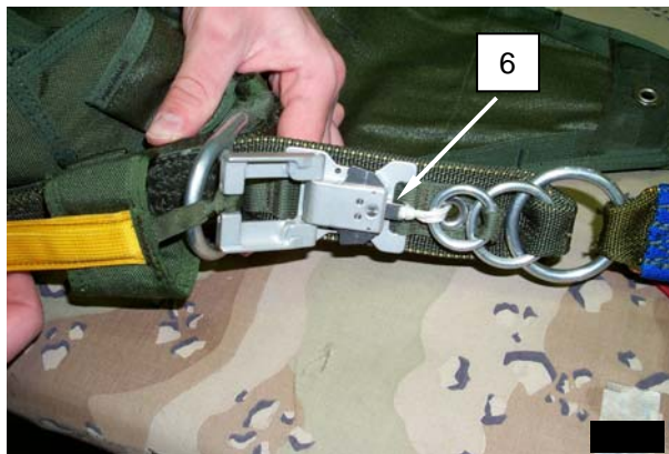
Figure 14. Inserting Locking Lug into Jaws of Canopy Release Assembly, Ensuring Locking Lug is Fully Seated, Close Canopy Release Cover, and Check Top of Lug.
