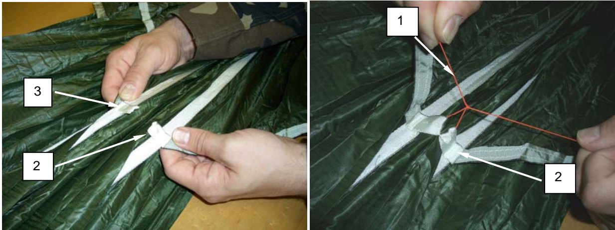
Figure 13. Tying and Securing Apex Scoop Loop Ends.
