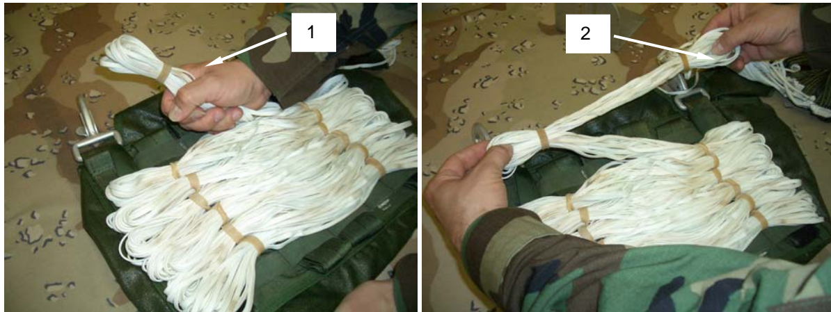
Figure 29. Forming Bight and Placing Retainer Band.
