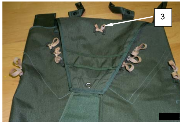
Figure 12. Attaching Large Retainer Bands on Static Line Stow Bars, and Small Retainer Bands Attached to Static Line Slack Retainer.
