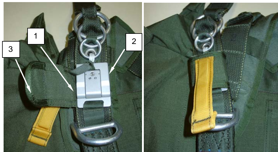
Figure 11. Inserting the Short and Long Tuck Tabs Behind the CRA.
