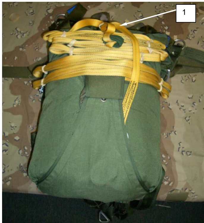
Figure 69. Stowing the 20-Foot Static Line.
