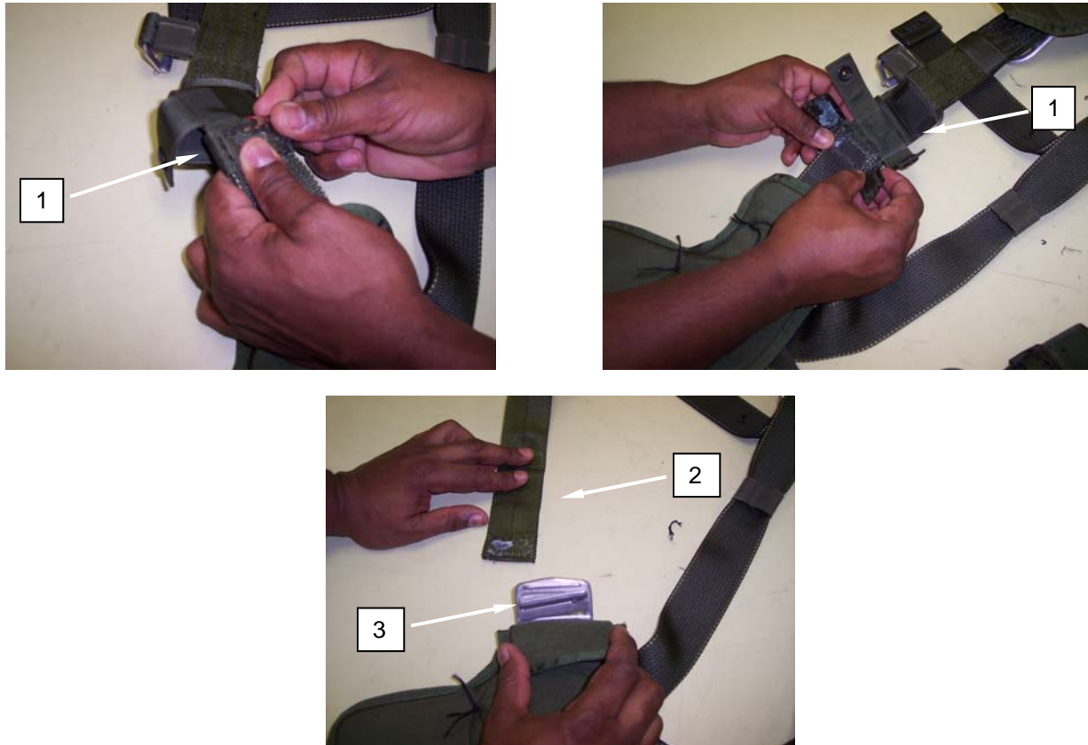
Figure 3. Replacing Harness Right Upper Main Lift Web (continued).
