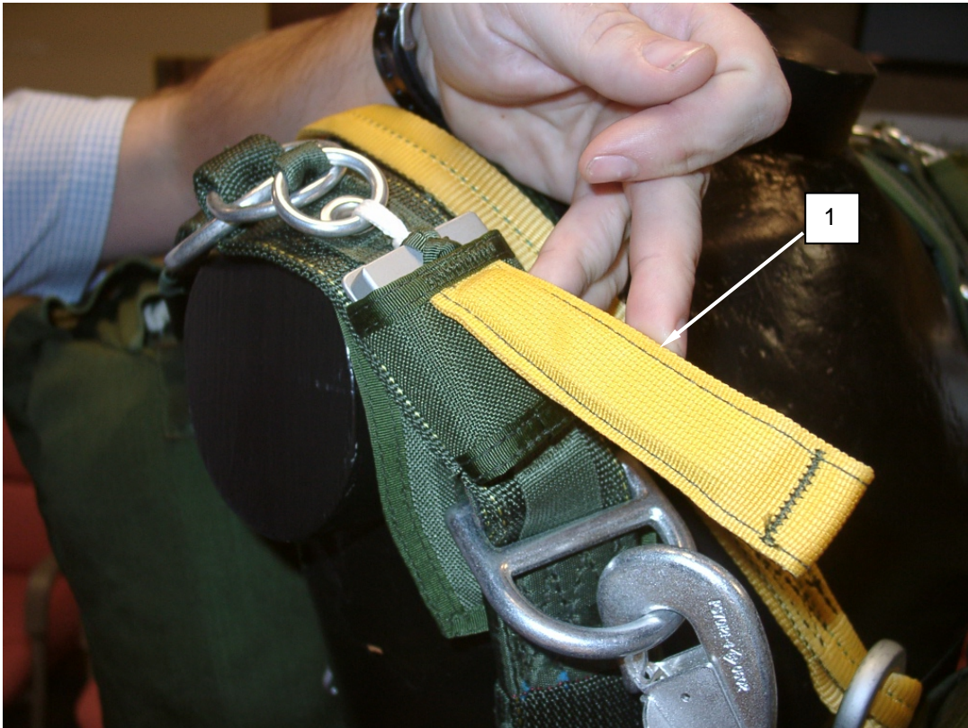
Figure 1. Open Canopy Release Assembly Cover Plate.
