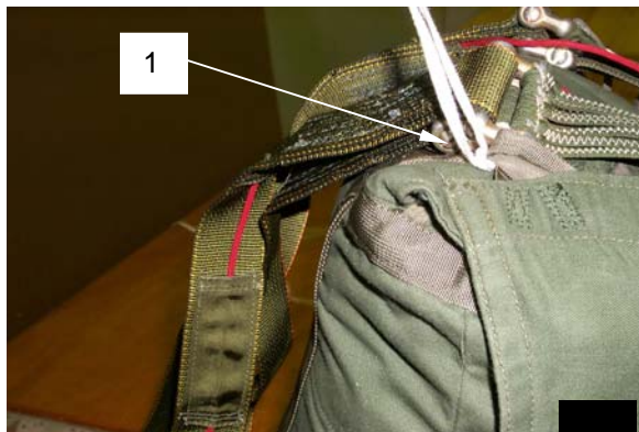
Figure 58. Tying Connector Links and Suspension Line Protective Cover (continued).
